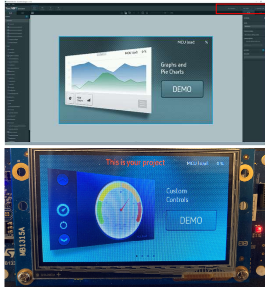
Flashing the project on the board from TouchGFX Designer
